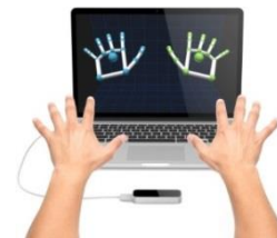
Fig. 2. The Leap Motion controller detects hands with infrared cameras. Then, hands are virtually modeled to control the computer.
